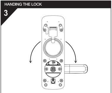
To hand the lock, on the inside of the handle, hold down on the metal slide tab -① located towards to bottom and rotate the handle left or right depending on your selected handing -②.
