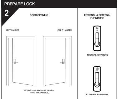
To prepare the lock for install, you will need to establish whether the door is right or left hand opening according to the image
