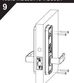
Taking care not to pinch the cables, fit the external lock body to the door.
