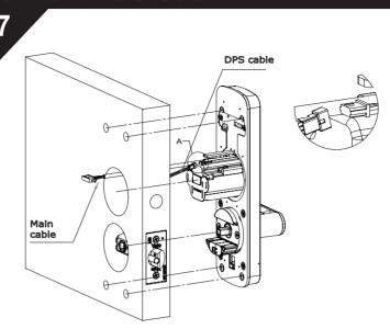
To fit the internal lock body to the door, feed the main cable and the DPS cable through the top hole and then fit the lock into place. Connect the DPS from the internal furniture to the DPS cable.
