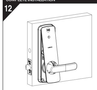
To complete the installation, replace the battery cover top end first and push bottom edge to lock into place.
