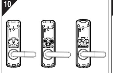
Push down on the battery tab as shown in the image to open the battery compartment. Install the 4 x AA Alkaline batteries.
