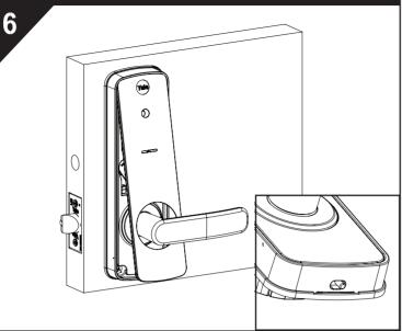
Remove the battery cover by the release tab located at the bottom of the internal furniture.
