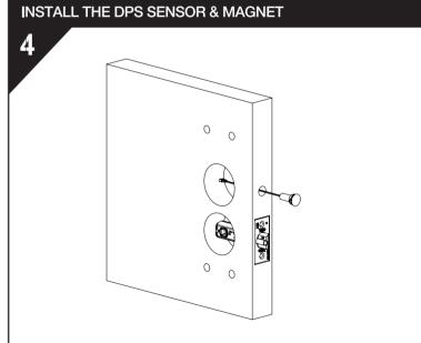
Insert the DPS through the 12.5mm hole on the dooredge. Feed the cable first through the DPS hole.
